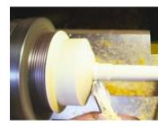
Paul then decided on the thickness of the stem and made a 'feature' transition at the bottom of the cup, leaving a shoulder at the top of the stem, then started to reduce the diameter of the stem to the desired thickness. He then decided on the shape and dimensions of the foot and created it. Paul stated that the diameter of the base needs to be approximately <sup>3</sup>/<sub>4</sub> that of the cup, when happy he turned off the lathe and unplugged it.
