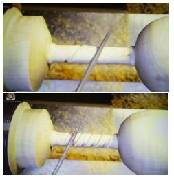
He laid the course cut file at 45\* to the stem at the base end, then by turning the lathe by hand he started to create a groove in the stem, he rotated the chuck as he was filing which starts to create a spiral groove in the piece, Paul continued in this manner until the groove met the top of the stem at the base of the cup.
