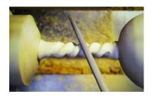
This system is repeated several times until the grooves are obvious and similar. Then he chose a different file and repeated the action to further define and deepen the twists. The shape, depth, and thickness of each twist can be altered and improved by use of the files and the angle of they are used. Continue the cuts until you are ½ the diameter of the stem
