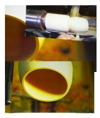
Paul stated that the goblets are usually about 31/2in deep and the same width, he initially used his 3/8 gouge with an "upside down" cut, then changed to his ball gouge to quickly remove stock from the inside. He again stopped the lathe frequently to check for wall thickness, ideally 3-4mm.
