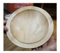
Richard then removed the piece and placed them in his 'Button-Jaws', adjusted the tool rest and by using a small bowl gouge he removed the inside recess and shaped the foot. When he was happy with the final shape, he finished off the inside of the base with the power sander to 320 grit, applied wax to the area and burnished it to his satisfaction. Richard states that he sells the finished bowl for £10-£12 at his Craft Fayres.
