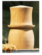
He then removes the tailstock to allow better access to the top of the hat and adjusts the tool rest, then shapes the top of the hat and removes the hole that has been left from the live centre and make a convex shape on the top. He then hand-sanded to 240grit, regularly stopping the lathe to check on the shape and tool work and clean-up, as necessary. Using a flat gouge Richard smooths off the bottom and gives a bit of shape to the 'body' of the gonk, and parts it off from the chuck.
