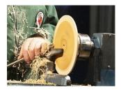
Richard then rotates the piece and starts to shape the front of the bowl, he always adjusts the tool rest accordingly, then using a 1/4in bowl gouge starts at the outside edge using push-cuts. He then changes to the smaller 'detail 'gouge' to shape the top outside edge of the bowl using both push and pull cuts. Again, he regularly stops the lathe to check for tear out and for 'low spots,' he then ups the speed to get a better finish on the lip of the bowl.
