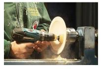
To assist with the sanding, Richard uses his power drill with a 'hook and loop' sanding pad with the lathe stopped. He also stated that he uses discount Baby-oil from the local Pound shop, which he sprays on and leaves for a few seconds to soak in, then he sands with 120-240 grit. The oily dust will gradually clog the sanding disc, but a quick brush with a brass wire brush will quickly clean it off, the disc can then be reused for a great finish.
