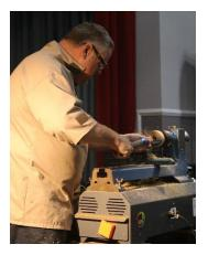
drill bit beyond the desired depth. He hollowed initially with a spindle gouge. Other than at the very centre, the tip of the gouge is not cutting - it will cause a catch. Instead, with the gouge at about "10 o'clock", the left wing of the gouge, near the tip, is doing the cutting. The wood was tearing out with this hollowing process. Sanding this away is difficult because the resin in the cedar clogs the abrasive.
