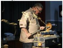
bowl. The technique was fun for the turner, as Les tried to cover the audience with shavings! The final ogee shape on the outside was cut from top to base because of the end grain material. A foot and chuck tenon were cut at the base.
