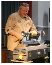
techniques for improving the finish. He began by roughing the blank to a cylinder, emphasising the importance of using a bevel rubbing cut and also of matching the feed speed to the lathe speed to give the tool a chance to cut. He said to advance the tool across the wood, never to push it. Angling the gouge to get a shearing cut will give an even better finish.
