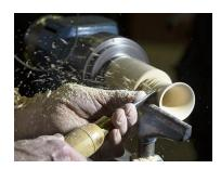
Mike was using gentle cuts to remove stock from the piece, and when he had removed enough, he used sandpaper with an 'artificial finger' (a piece of wood which Mike had attached a rubber tip with Velcro wrapped around it and attached some hook and loop sandpaper) which he can safely insert into the narrow opening of the goblet's mouth, and using different grit paper to achieve his desired finish, and moving the tool rest closer so that he can safely support the tool.
