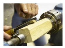
He attached his Spalted Beech blank to the lathe via live centres and turned a shoulder for the tenon. Mike then inserted the 'tenon end' of the blank into the chuck and pulled-up the tailstock to hold it securely and turned the whole piece to 'round' and used a smoothing cut to make the end smooth. Mike then made a small indent into the centre of this end and uses is as a start point to make a hole with a drill, this is the start point for the hollowing out as it
