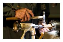
With the wire cut to the correct length and shaped to round. He placed the wire over the 'trench' and offered up the Tail stock to give the blank some support,
