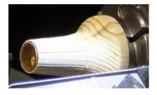
and securely and allows free access to the inside face of the ring. Mike sanded the inside to gently curve the ring. When he was happy with the front edge, he removed the ring and inserted it the other way round so thet he could shape the other inside edge, paying particular attention to getting both inside faces the same.
