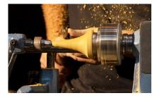
same size as the dowel into the end and rotated this piece so that the tenon with the hole was held in the chuck and started to shape the hat into a broad-based cone with a bobble on the top. When the shape was as desired, Tom sanded it to a fine grit and sealed it. Normally he would finish to a high gloss to enhance the overall appearance of the Gonk but due to time limitations he just left it sealed.
