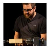
cuts towards the middle of the spindle to reduce tear-out at the ends and turns the blank to round. He then turns the lathe to full speed to get a smooth finish and puts a chucking point on both ends of the blank using callipers which had been adjusted by welding small washers onto the tips to prevent any dangerous catching, as designed by Mike Haselden.
