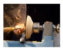
3cm in from the edge and a second mark 8cm in from the first mark and proceeded to remove the stock between the lines to a depth of 3mm to make a trench.
