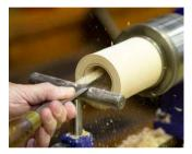
The base was hollowed out to the planned depth by using different sized gouges, and the body was then shaped. The lid was then turned and formed to the planned shape and attached to the body.
