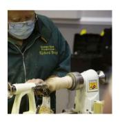
The lid, when turned and shaped was a very good fit and was sanded and waxed using Chestnut Cut-n-polish.
