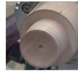
will then house a small jewel, later in the process. To finish off the inside of the lid, Cindy reduced the speed of the lathe and used a negative rake scraper to give a better finish and then sanded using 400, 600 grit paper and then finished with Abranet mesh. When it comes to finishes, Cindy uses cellulose sealant sealer, this will 'pop' the grain. She uses this as it keeps the wood a light colour; She used Krylon spray finish
