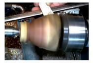
shape and so lengthened and flattened it. To get a good finish, he could have used a scraper, however he prefers to use a skew chisel as a negative rake scraper. He pointed out that some species of wood are better than others for scraping. Colwin put some more CA (thin) glue in the cracked centre.
