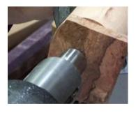
'fault' would not be part of the inlay. Cindy used a 1/8" parting tool to turn the inlay to round, then then measured the inlay with vernier callipers and scribed this onto the end piece.
