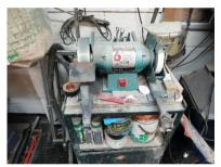
to reshape profiles or sharpen really blunt tools. I could not recommend using CBN wheels for sharpening enough, I have had the same wheel for over 3 years now and it is still going strong. I have made my own sharpening jig with attachment for sharpening my tools, making sure I can achieve an accurate repeatable grind. I have made a video on making and using this system on my YouTube channel:
