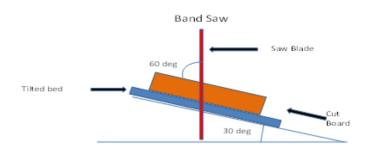
When you set the band saw bed at 30deg, the cut you get is 60 deg. As you can see from the diagram above the blade remains vertical whilst the wood is tilted on the bed. I hope I am not boring you, but I made a mistake by just adjusting the band saw bed without checking the consequences. The result was the rings would not stack, and I could only use every other cut ring. So, it was back to the pencil and paper to solve the problem.
