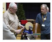
Lathe 5 With Alan Sturgess, Alan started by showing how to 'face-off' the blank in order to stop the vibrations caused by the unsymmetrical wood blank and then commenced the shaping of the bowl they
