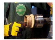
He then started to sand the Bangle with 60 grit sanding paper, sanding the inside as well as the outside. Once the wire was semi-circular, he then went up the sanding grits e.g. 180. 240, 320, 400
