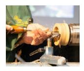
to the Lathe bed. He then used a round scraper to remove some of the waste block (on the inside); this is to aid sanding the Bangle later in the process.
