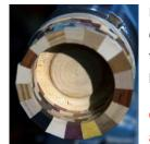
He uses an extra wood piece on the opposite end of the waste wood and then clamps the pieces together and leaves to cure overnight.
