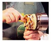
he puts some glue in a portion of the slot and then puts the copper wire in and pulls it tight by pulling on the electrical block and by using a spare piece of timber to push down on the wire in to the groove, ensures it is sitting correctly; he spayed accelerator on the glued portion to speed up the drying time.
