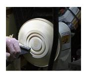
remove the necessity of flattening the base after the spigot is removed. Alan demonstrated his method to the team. With the bottom finished, and the bowl reversed on the chuck it soon became apparent that the knot was going to cause an issue. Mike decided to pour some superglue into the hole to stabilise it and then carefully proceed with the hollowing. The glue held and the bowl was sanded to satisfaction then sealed with spray
