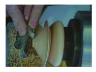
Another quick demo was to make balls from small offcuts of burr oak. Jason makes a lot of these for solitaire sets and they must be done quickly to a uniform size. Mounting the wood
