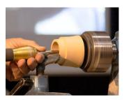
Les swapped out the lid for the base and then trued the end. Once completed he then started to hollow out the bottom in an egg cup shape; he mentioned that you could use a bowl gouge with a pull
