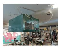
micron to 5 microns. This dust in the air can cause long term damage over a long exposure period as they are not blocked by the mucus membranes in your lungs. It has a timing feature which allow me to leave it running for a few hours after I've left the workshop to filter out the air. I normally use a JSP IP powered respirator whilst turning to protect my face and lungs,
