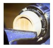
Les then returned to the pull cut to finish the hollowing, and used the universal tool to square the sides and the bottom of the lid
