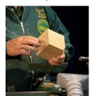
be safely held on the lathe by a Steb Centre, the opposite corner is supported by a 'live Ring Centre' in the tail stock.
