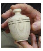
The foot of the base was then shaped to his satisfaction, sanded and sealed, then fine sanded with 400 grit with a finishing coat of Cut and Polish to finish. The Parting Tool was then used to separate it off but leaving enough to make a 'Jam Chuck'. The completed Lid and Body of the box were then taped
