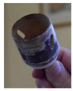
between centres, it was turned to a cylinder of the required diameter, marked with a length equal to the diameter and the ends turned to make an approximate ball. Jason then used a hole cutter of suitable diameter, sharpened at the end, moving against the revolving ball to shape a perfect sphere (although
