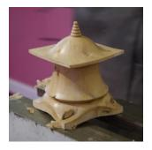
the lid and at the bottom of the base where it is fashioned into 4 feet. Much of the cut is through air and if not properly controlled the tool will bounce when it meets the corners. The bevel has nothing to rub on. A sheet of white paper on the lathe bed
