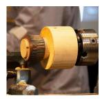
project; Les removed the spigot without the tailstock in place, removing the spigot in multiple passes and finished with the micro bevel which will give the best possible finish on end grain,
