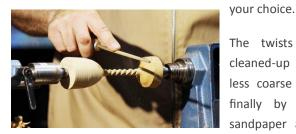
The twists can be cleaned-up by using less coarse files and finally by wrapping sandpaper around a
