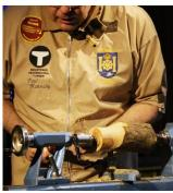
Paul's demo was "Making a Goblet" and for this he had chosen a 12 inch piece of branch-wood Yew, the piece had a few 'shakes' on one end and a small split and a branch knot on the other, he chose the end with the 'shakes' to be the base of the goblet, any splits or shakes on the 'cup' end of the goblet would have weakened it.
