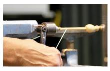
He then parted the piece from the lathe inserted the tail into the hole 'caught the elastic band' and gently pulled it out,
