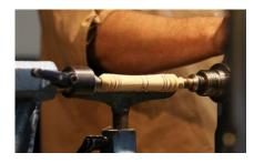
The second part of the Idiot Stick is made from a similarly sized piece of OAK that is placed between centres and turned to round then reduced
