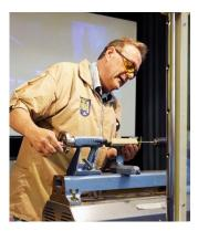
Whilst supporting the piece of Ash in his hand he continued to drill through three quarters of the length of the blank by slowly pushing the piece into the drill which was spinning at medium speed. This is a perfectly safe method of completing a hole by hand and it ensures that
