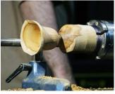
Before turning too much wood from the stem Paul placed a tennis ball sized polystyrene ball inside the cup and held it in place with the tailstock to support the fragile cup whilst he removed wood with the gouge by pulling towards the chuck end to prevent tearing the fibres.
