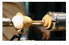
stem was blended into the cup and the base turning coves and ogee shapes grooves to create a pleasing overall shape
