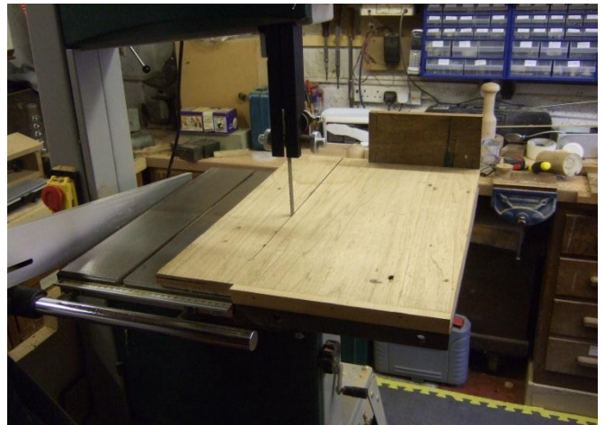
Stop bar and upstand showing the saw blade having cut a slot down the plate.
