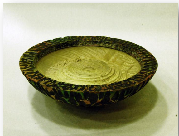
Ash bowl, textured and stained ready for centre to be hollowed.
