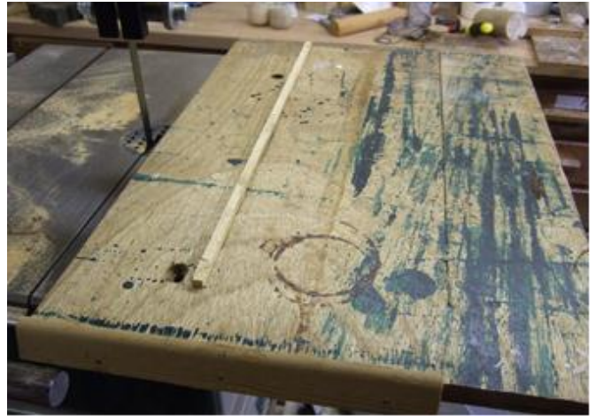
The underside of the jig showing the batten strip that slides along in the channel of the metal table plate.
