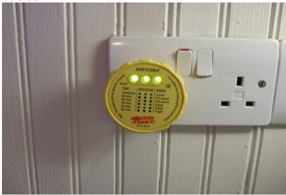
A plug in tester showing a good Earth and Line & Neutral are connected correctly. Plug in testers are available from all good electrical and DIY stores at a cost of around £8 - £10.
