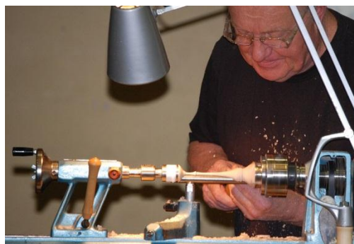
Turning a spindle under tension
