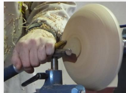
Pull cuts and push cuts with the versatile long grind gouge
