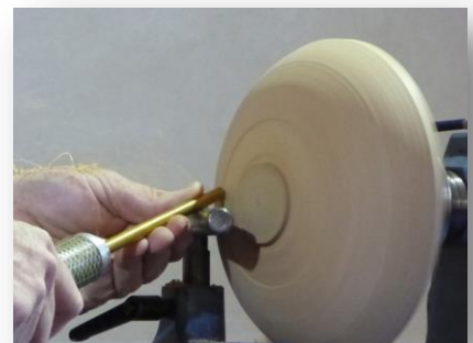
Pull cuts and push cuts with the versatile long grind gouge
