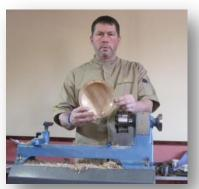
His first demo was of a bowl made from one inch timber turned to a fine finish to demonstrate the turning techniques using a bowl gouge.
