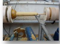
The bowl and foot are clamped in wooden chucks at the head and tail stocks. Tension is applied before turning the stem very thin.
