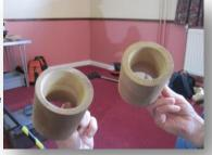
The inside was hollowed to give a taper to suit the object to be held and different sizes can be turned on either end of the chuck.
