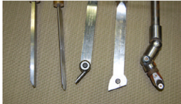
The picture shows some of the tools demonstrated. From the left they are the "hardwood scraper", "spindle master", sheer scraper with hollowing tip, sheer scraper with scraper tip, the "Ultimate" hollowing tool
