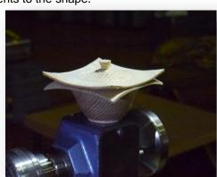
He uses a 50/50 dilution of cellulose sanding sealer, applying multiple coats with an air brush rubbing down in between.
