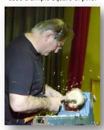
Kevin started the first half of his demonstration with the base of the box using a faceplate ring inserted in the collet chuck, very similar to turning a bowl but taking care when shaping the square edges or wings. This was then reversed onto the chuck for hollowing out.
