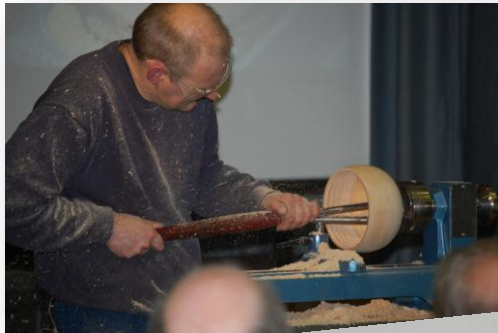
Steve hollowing his bowl and the groove cutting tool
