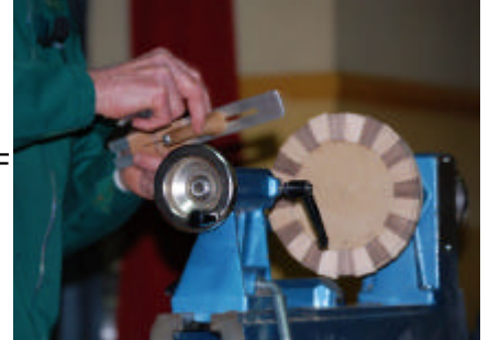
MDF disc with alternating segments for inlay. Note marking up jig
