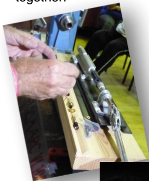
Pen parts being assembled on Miles Craft press jig.
