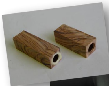
Divided blank with tubes glued in, left and Ron turning the pen assembled on mandrel, below
