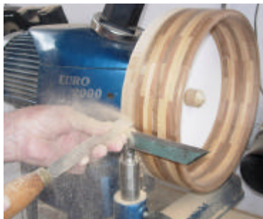
Turning the cylinder made up of segmented rings
