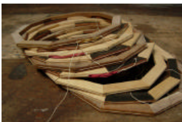
A set of rings, above, held together with strings and, right, assembled ready for turning.
