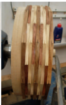
A set of rings, above, held together with strings and, right, assembled ready for turning.
